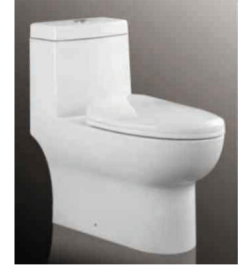
T138 * Vitreous china * Siphonic one piece toilet * Low-consumption(6.0/1.6gal) * S-trap, single hole water outlet * Slow down cover plate, Bange
